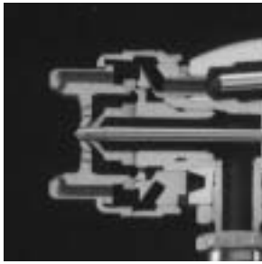
BALL / CONE SEATING ENSURES CONCENTRICITY OF THE AIR CAP TO THE FLUID TIP
